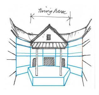
Fig. ? (a) Stage, tiring house and Gentlemen's rooms ('Lord's room) cordoned off and raised above the level of the ajoining galleries
