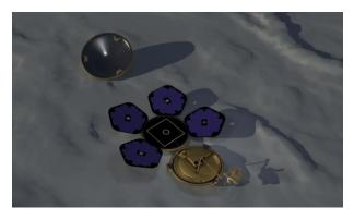
Figure 3: Lander with four panels and robotic arm deployed, heat shield and terrain (WIP render)
